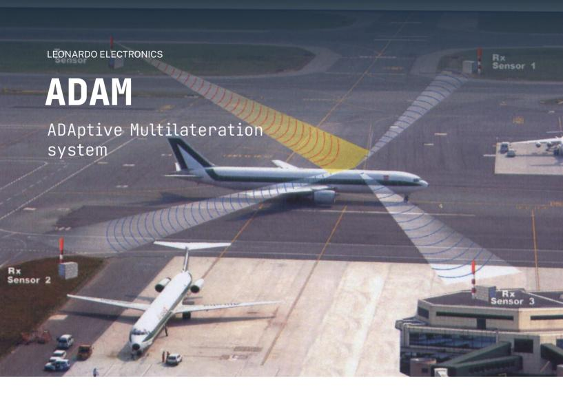
ADAM (ADAptive Multilateration) is the Leonardo Multilateration system for accurate all-weather surveillance for Airport and Wide Area applications. ADAM exploits outstanding advanced sensors design and innovative target processing in a flexible and redundant architecture tailored for co-operative targets moving on the airport surface. ADAM can be employed as well for TMA/En-Route airspace surveillance.
