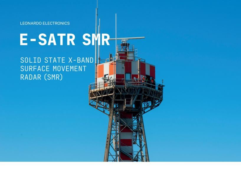
The SMR Enhanced Surface Airport Tracking Radar (E-SATR) is an X-Band, state-of-the-art, solid-state, high-resolution radar for complete ground movement control in A-SMGCS systems. It has been developed in accordance with EUROCAE MOPS and ICAO requirements for performance and integration purposes in A-SMGCS systems.
