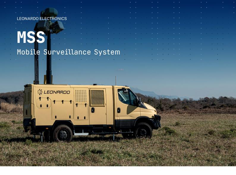
The MSS is an high mobility vehicular integrated system for on field surveillance which includes radar sensors, an optronic system, a Command & Control and Communication facility. The components combined performances allow the system to detect air, ground and maritime targets up to the nominal distance of 40km.
