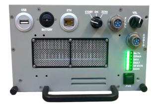
The CCR is a new generation, multi-band and multiprocessing module specifically designed to extend the capabilities of the land and airborne Swave SDR family to the naval communications domain. The CCR accomplishes the following main tasks:
