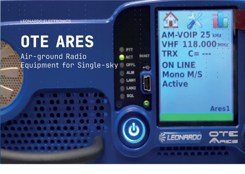
OTE ARES (Air-ground Radio Equipment for Single-sky) is the 5<sup>th</sup> generation of VHF and UHF radio equipment family. Thanks to its software-defined radio architecture, conceived with a new design concept, the latest Leonardo radio equipment series can be used for transversal system solutions, suitable for both ATC and Defense markets.
