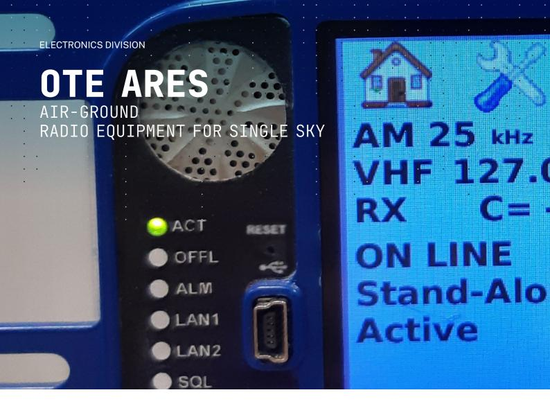
OTE ARES (Air-ground Radio Equipment for Single-sky) is the 5th generation of VHF and UHF radio equipment family, representing the top quality Leonardo product line for ground-to-air civil and defense communications. Thanks to its software-defined radio architecture, conceived with a new design concept, the latest Leonardo radio equipment series can be used for transversal system solutions, suitable for both ATC and Defense markets.
