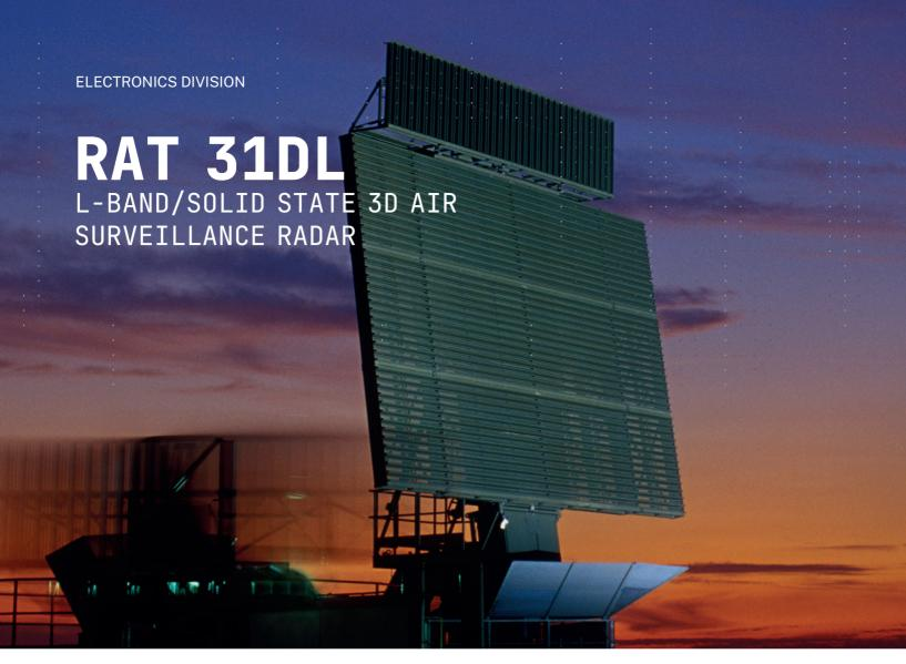
The RAT 31DL is an advanced L-band solid state active phased array, 3D surveillance radar, effective to a range of over 500km.
