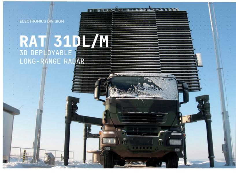
The RAT 31DL/M is a tactical deployable Air Defence long-range radar operating in L-Band. Designed from advanced Air Surveillance requirements against ABT and TBM threats.
