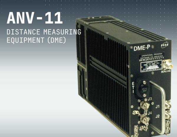
Among its CNS solutions, the company provides the ANV-211 DME/P (Distance Measuring Equipment Interrogator/Precise), capable of receiving accurate distance information from DME/P Transponders and standard distance information from conventional DME/N Transponders. It meets the requirements specified in the RTCA-DO/189.
