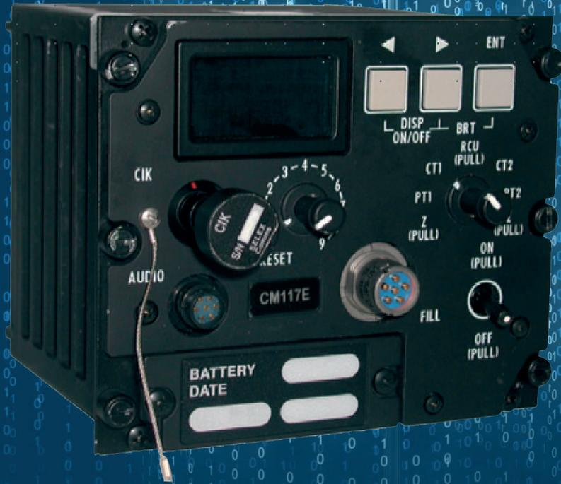
CM117E device is a multiprotocol data and voice encryptor for airborne, land and naval tactical applications. It operates in narrowband or wideband modes, interconnected to either HF, VHF/UHF radios or wired lines.
