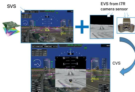
SLAD-208 provides all typical Electronic Flight Instrument System (EFIS) functionalities like Primary Flight Display (PFD), Electronic Horizontal Situation Indicator (EHSI) for Navigation Display (ND), Engine Indicating and Crew Alerting System (EICAS); optionally a Flight Management System (FMS) can be integrated.
