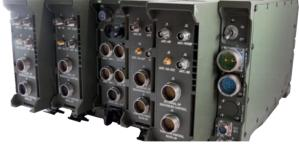
The unit supports the more advanced state-of-the-art Mobile Ad-hoc Network (MANET) waveforms as ESSOR HDR, S-HCDR and SelfNET® family, composed by by EPM/ ECCM EASY II, NarrowBand Adaptive Waveform (NBAW), Soldier Broadband WF (SBW) and the emerging NATO Narrow-band.
