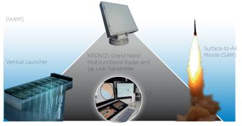
multilayered defence system, such as a combat system, providing the following operational advantages: Shortest reaction time for track initialization. After the initial detection of a new threat, KRONOS® Grand Naval confirms the threat in the same rotation scan, initializing the track within the next mechanical scan. This capability is essential against pop-up targets, such as Sea Skimmer missiles and helicopters. Shortest reaction time for both tracks cueing and engagements
