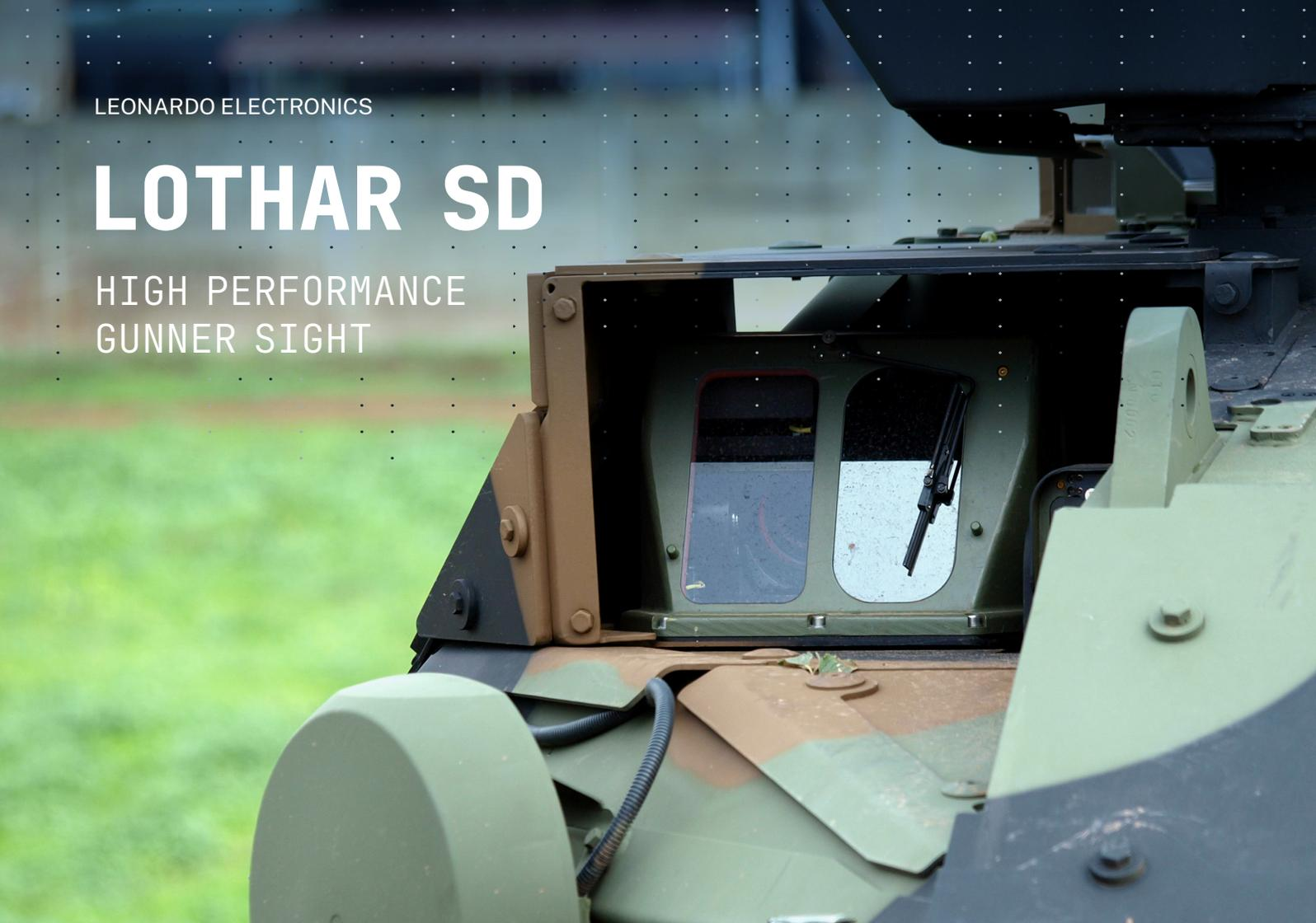
LOTHAR Stabilised Digital is a two axis gyro-stabilized gunner sight designed for high-accuracy target engagement and fire on-the-move during day and night at all combat scenarios and all weather conditions.
