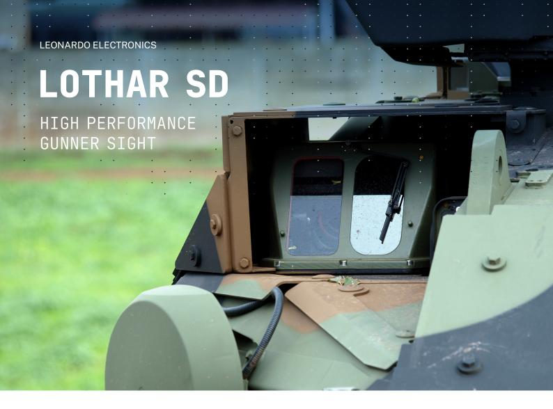
LOTHAR Stabilised Digital is a two axis gyro-stabilized gunner sight designed for high-accuracy target engagement and fire on-the-move during day and night at all combat scenarios and all weather conditions.
