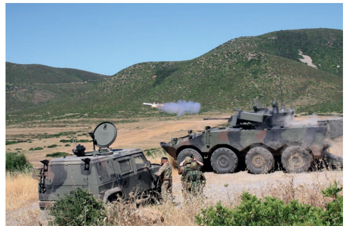
The HITFIST® 25 mm turret in anti-tank configuration installed on the VBM Freccia of the Italian Army, during SPIKE ATGM launching test
