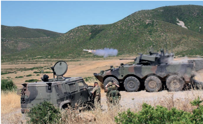
→ The HITFIST® 25 mm turret in anti-tank configuration installed on the VBM Freccia of the Italian Army, during SPIKE ATGM launching test
