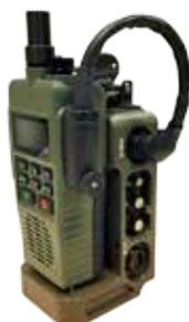
The **SWave® VM3** is a vehicle variant of the company's Hand Held single-channel SDR. It has been designed for those vehicular applications where a single channel radio is sufficient to cover the vehicle communications needs as well as provide the necessary link to dismounted soldiers. The radio operates in the 30MHz to 512MHz frequency range and supports both legacy and new waveforms in VHF and UHF frequency bands.
