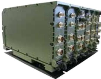
The **SWave® VQ1** is a four-channel vehicular radio that provides secure voice and data services for current and future tactical communications needs. The radio features a modular HW architecture that allows up to four radio channels to be configured within a common chassis with a shock mounting base.
