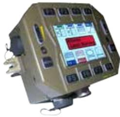
The **UIS-379/D** allows very reliable communications, in addition to others services such as wireless connection between crews, voice and video recording and data terminal connection based on IP Network technology. UIS-379/D has a distributed and modular architecture with units connected via a digital serial bus.
