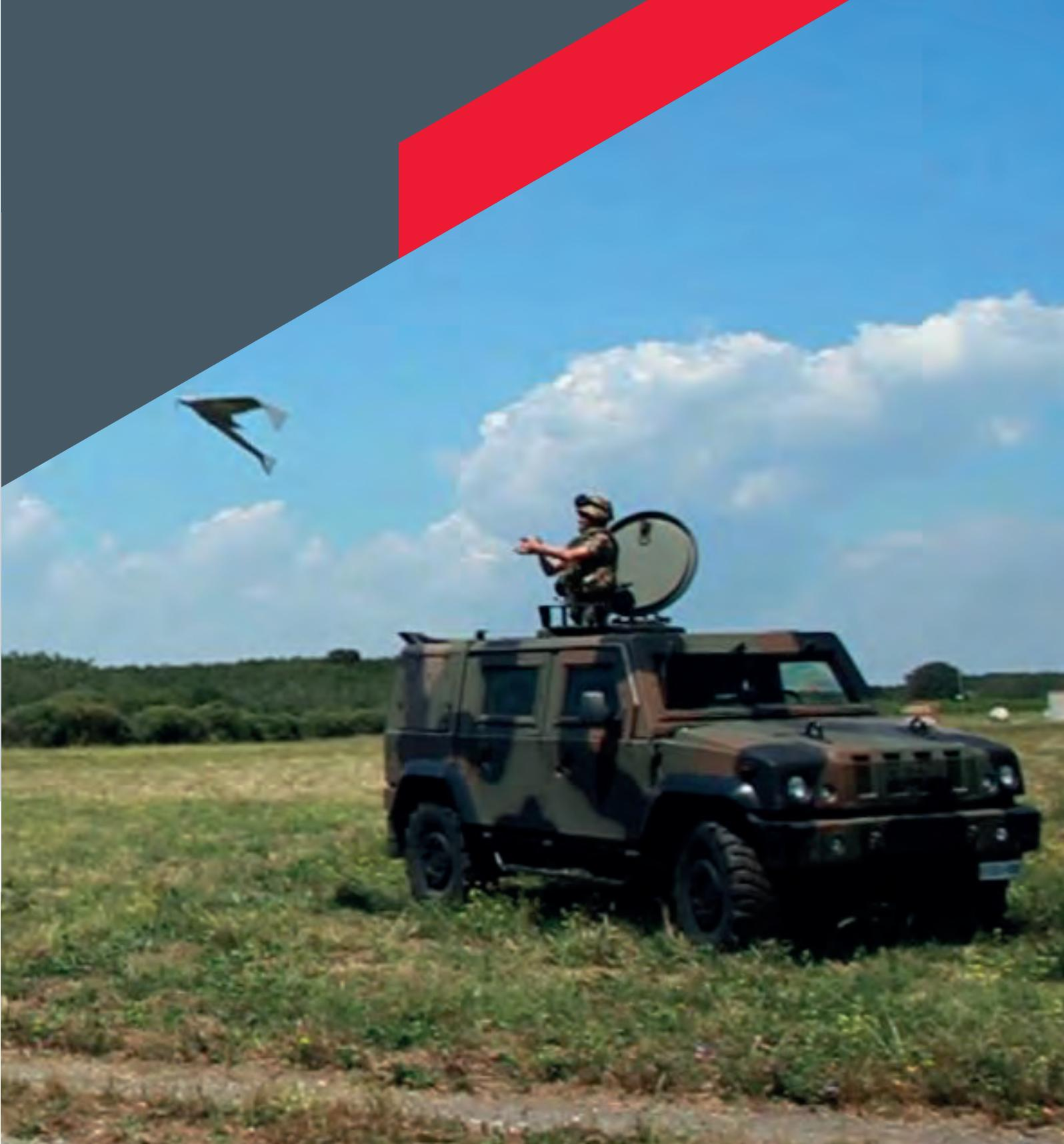
CREX-B is a fixed-wing, electrically powered UAS with endurance of over 70 minutes. It can be hand-launched from enclosed spaces by a single operator, without the need for run-ups. The system can be transported in a back pack and operated by a single operator.
