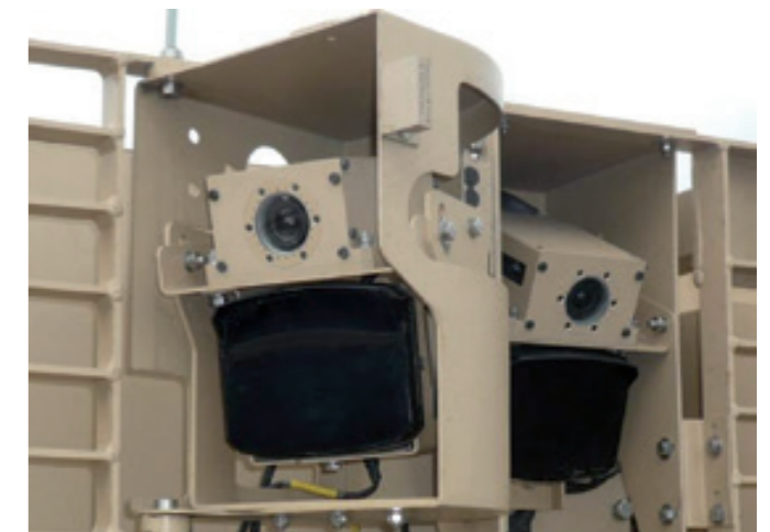
Typical Camera and IR Illuminator installation
