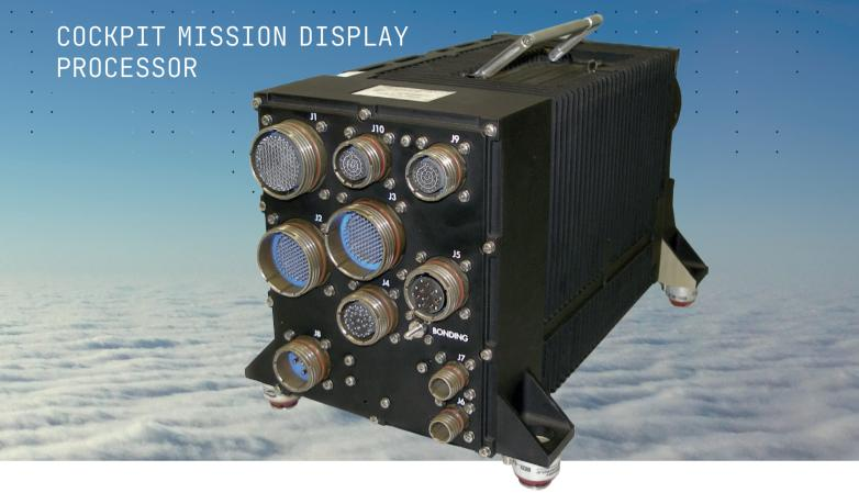
The Cockpit Mission Display Processor (CMDP) is a high safety avionics computer platform with a powerful embedded graphics capability. It is configured using the base of the standard hardware and layered software modules, both developed by adopting the latest quality standards that make the CMDP certifiable according to D0178B and D0254 level B (optionally level A) and suitable as a main cockpit mission computer.
