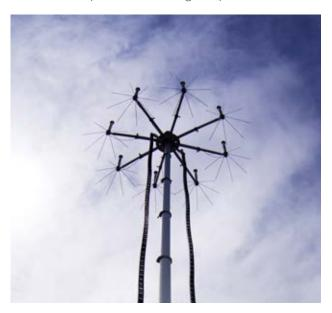
Passive radar systems are unique because they do not have their own transmitters but exploit the electronic waves already produced by existing sources e.g., FM radio signals, telecommunication equipment. Passive radar systems are often referred as Passive Covert Radar (PCR) and, as a covert radar, the system is ideal for military applications.
