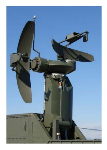
During the installation phase the platform is lifted to the final position by the motor driven movable central arm (Lifter). The arm permits also the placement of the platform to a convenient height for the installation/maintenance of both antennas.
