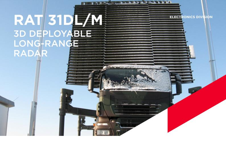
The RAT 31DL/M is a tactical deployable Air Defence long-range radar operating in L-Band. Designed from advanced Air Surveillance requirements against ABT and TBM threats, it has been delivered to many countries around the world, including a number of NATO members.
