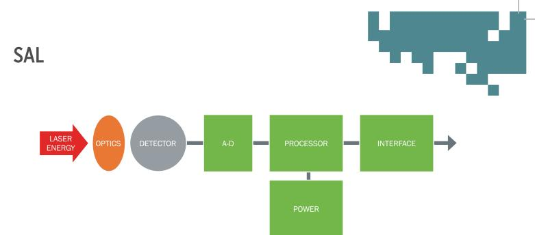
The GEN III SAL seeker product uses a unique configuration silicon detector providing continuous high resolution angular reporting over a wide field of view. Configuration of this technology is the subject of patents both granted and under application.
