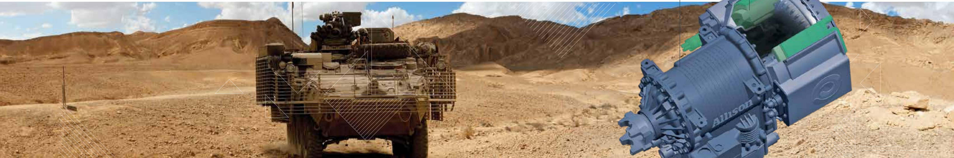
The Transmission Integral Generator (TIG) features a Leonardo DRS generator combined with an Allison military transmission.
