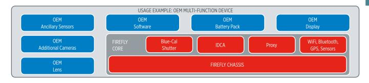
The presence of two additional camera channels allows Firefly to be used as the core of a multi-waveband imager. Combining multiple camera channels into one processing core allows image fusion and provides net SWaP-C savings. The combined software and hardware power management system allows Firefly to offer state of the art power efficiency.
