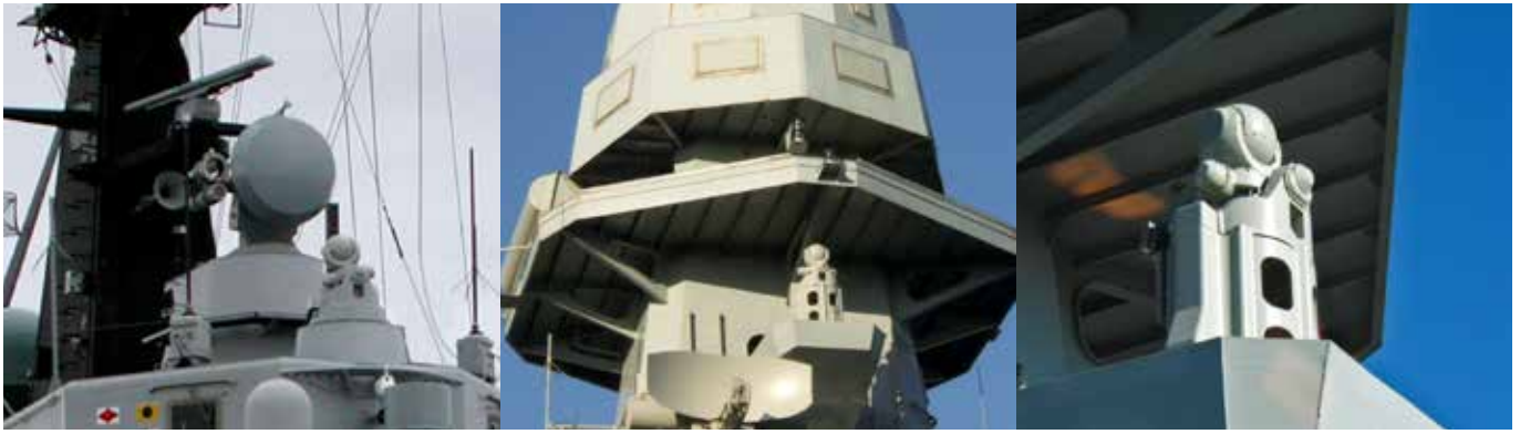
SASS installations on-board Euro Maestrale (1) and NUM Cavour (2-3)
