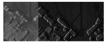
Comparison between a true 90° Spotlight Doppler Beam Sharpening (SpDBS) image (left) and the corresponding real-time MARS simulation (right) using FFT processing (2 meters resolution on the Oberpfaffenhofen airport).
