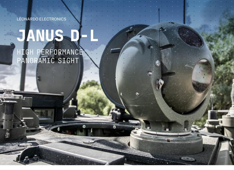
JANUS Digital-Land is a modular dual axis gyro-stabilized sight for MBTs and AFVs, designed for day/night panoramic surveillance and target tracking in a rugged and compact suite. Being able to aim up to +70°, the sight is suitable also for urban scenario against high elevation targets.
