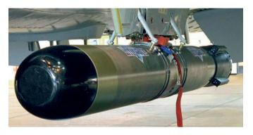
The inertial system exploited for the torpedo control and guidance is based on 'strap-down' technology providing the weapon with an excellent manoeuvrability, all-attitudes capability including bottom following capability and high accuracy for the final impact on the target.
