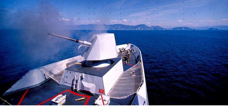
The OTO 76/62 Super Rapid (SR) Gun Mount is a light weight, rapid-fire naval gun providing unrivalled performance and flexibility in any air defence and antisurface role, particularly in anti-missile role.
