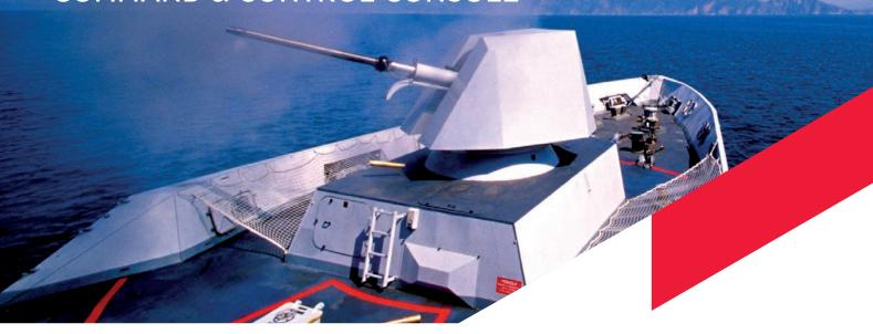
The OTO 76/62 Super Rapid (SR) Gun Mount is a light weight, rapid-fire naval gun providing unrivalled performance and flexibility in any air defence and antisurface role, particularly in anti-missile role.
