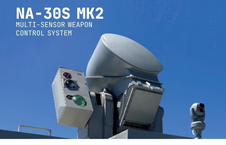
NA-30S MK2 is a new generation Weapon Control System designed to control modern guns (up to three) against conventional and asymmetric air/surface threats with a reduced reaction time.
