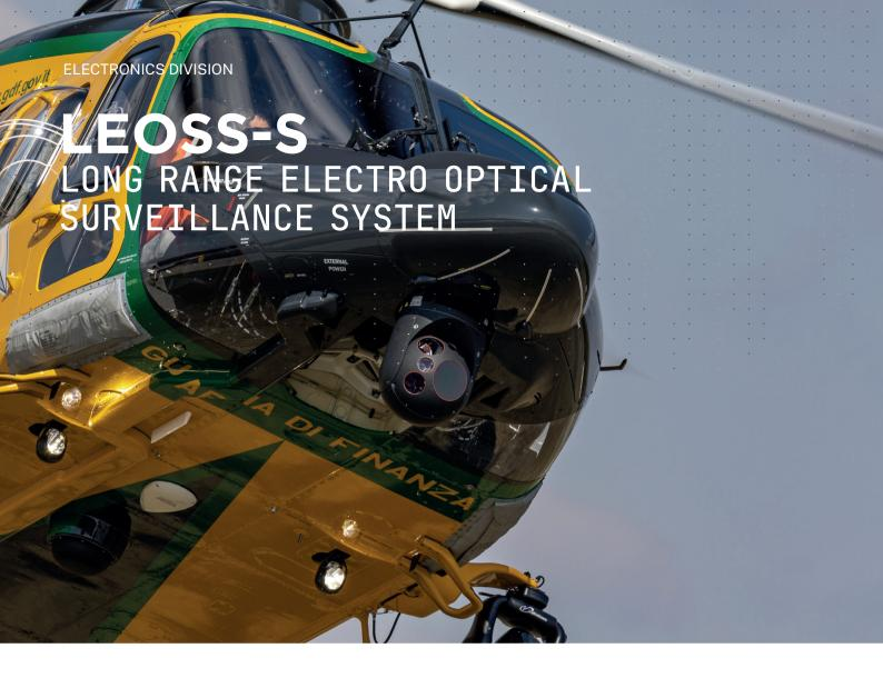
LEOSS-S is the latest multi-sensor, high accuracy, 4 axes gyro-stabilised turret system designed for airborne surveillance applications.
