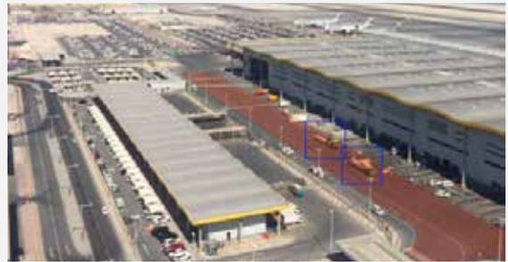
**Anomaly detection Step 1** Take the reference image of the area to be monitored (it can be auto updating according to a specified rate)
