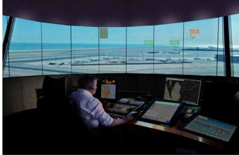
Whilst the initial focus has been given on day-time VMC operations, nocturnal and low visibility operations can also be supported by means of additional sensing equipment, infrared or night-vision cameras and three dimensionally-augmented reality overlays.
