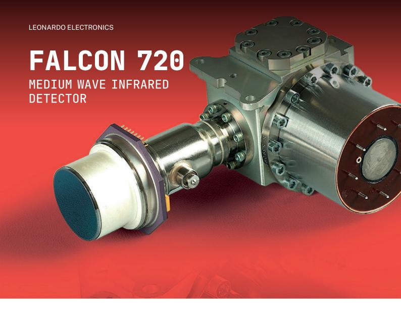
The Falcon 720 infrared detector uses the latest focal plane technology to provide high definition infrared images compatible with commercial 720p HDTV signal formats. The  $12\mu m$ -pitch focal plane array enables this high definition detector to be offered in a compact, low-cost, low-power format.
