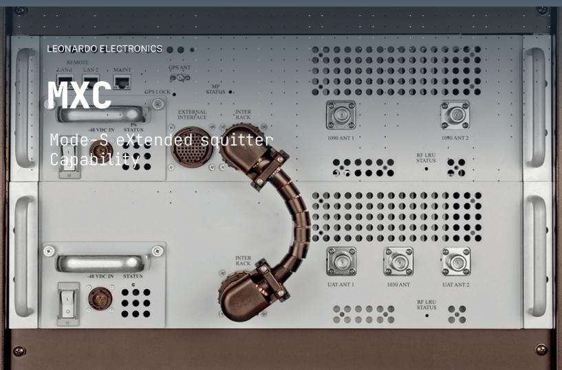
MXC (Mode-S eXtended squitter Capability) is a high performance ADS-B (Automatic Dependent Surveillance Broadcast) Ground Station for en-route, approach, and airport surveillance applications compliant with the 1090 MHz Mode-S Extended Squitter standard.
