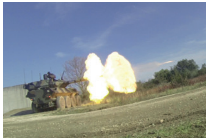
Firing capability in any position even on sloping terrain thanks to the low recoil FORCE cannon
